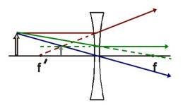
8. Construct the image on the drawing below via ray tracing.
